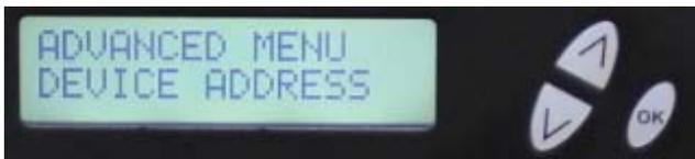
5. Set a unique Device address for each encoder being installed in the system.
