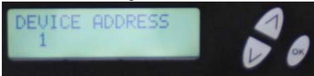
**Warning: Setting the “DEVICE ADDRESS” to 0 will clear the network setting to the Factory Default value.**
